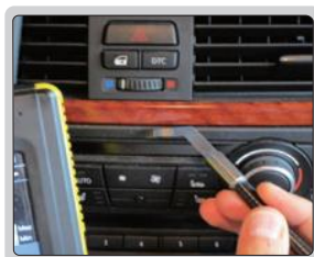
measuring gaps on the car dashboard
