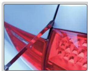
measuring car body seam
